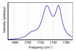
This spectrum was taken of a solution of two liquids. Three peaks are clearly visible: two strong peaks around 1750 cm<sup>-1</sup> and 1730cm<sup>-1</sup> and a weaker peak around 1710 cm<sup>-1</sup>. Given the molecules present in the sample, however, only one peak is expected in this area of the spectrum (the C=O stretching region). We observe multiple peaks because the molecules absorbing light are switching between three different environments!
